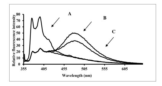
**Figure 3:** Excitation and emission spectra of the terminally located probe system (**A**) 3'-pyrenyl and 5'-pyrenyl probes (**B**) 3'-pyrenyl+ 5'-pyrenyl in 80% TFE/0.01 M Tris, 0.1 M NaCl, pH 8.4) at 5 °C with wild type target and (**C**) 3'-pyrenyl+ 5'-pyrenyl in 80% TFE/0.01 M Tris, 0.1 M NaCl, pH 8.4) at 5 °C with mutated type target (SNP). Component concentrations were 2.5 µM (equimolar).
