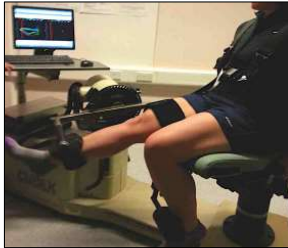
Figure 1: Isokinetic knee moment assessment
